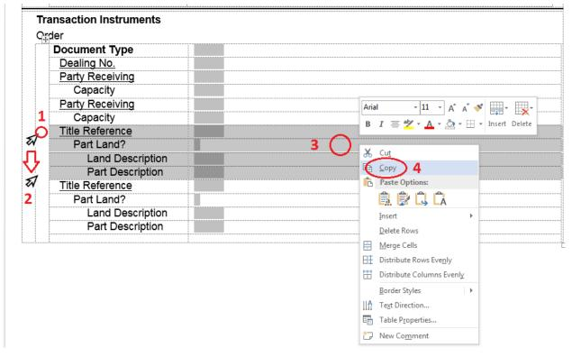
Place the cursor to the left of the row which the empty fields are to be inserted above so that the mouse cursor is oriented to the right ( $\vec{x}$ ) then left click to highlight the row (1). Right click within the highlighted row (2) to show the menu and select Insert as New Rows (R) (3).
